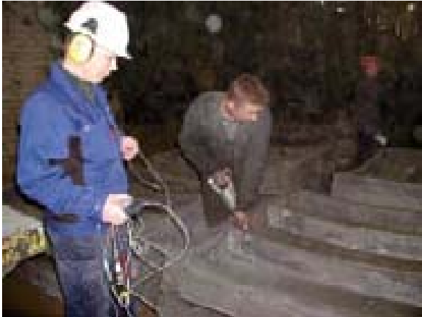
Photo 4. Noise dose measurement in maintenance department
