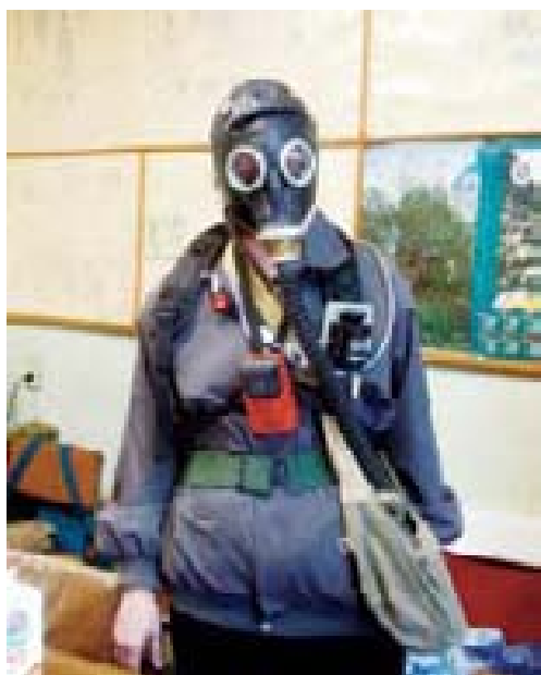
A worker equipped with personal sampling equipment. Nickel carbonyl Department, Monchegorsk Nickel refinery
