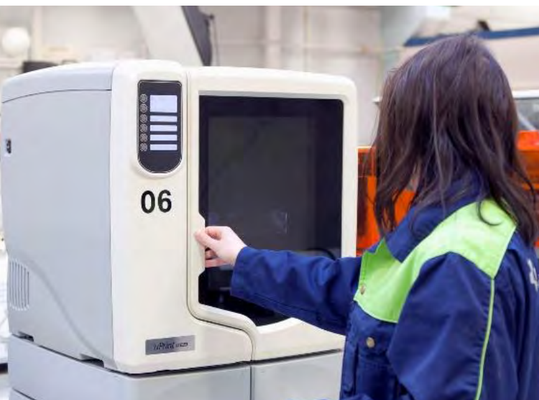
IMAGE. An enclosed printer reduces the spread of pollutants
